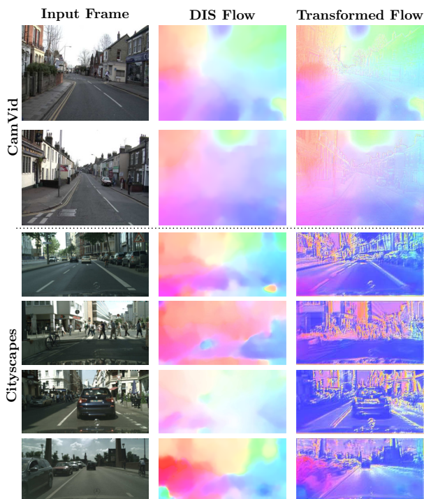
Figure 5. Effect of flow transformation. Example results of input and transformed flow, after training for semantic segmentation. There is a qualitative difference between CamVid and CityScapes. Best viewed on screen.
