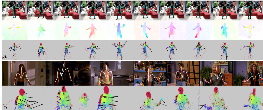
Fig. 4: a) Smartphone FlowCap. Here the video is captured using a hand-held phone camera. This results in overall flow due to rotation and translation of the camera. Despite this, part estimates remain good and pose is well estimated. b) Archival video. Results on archival data from series Friends and Buffy. Ground truth shown in red, [27] in yellow, FlowCap part centers in white.
